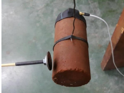
Fig. 5: Generating of Shear Waves in FFR Test.
