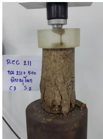
Fig. 7: A Photograph of UCS Test of a Pavement Recycling Material with 3% Cement Ratio.
