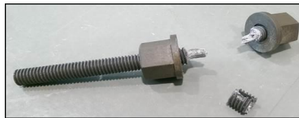
Fig. 5: Shear failure in FB10.
