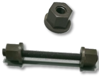
Fig. 1: Photo of the FRP bolt, washer and nut used in the experimental program.
