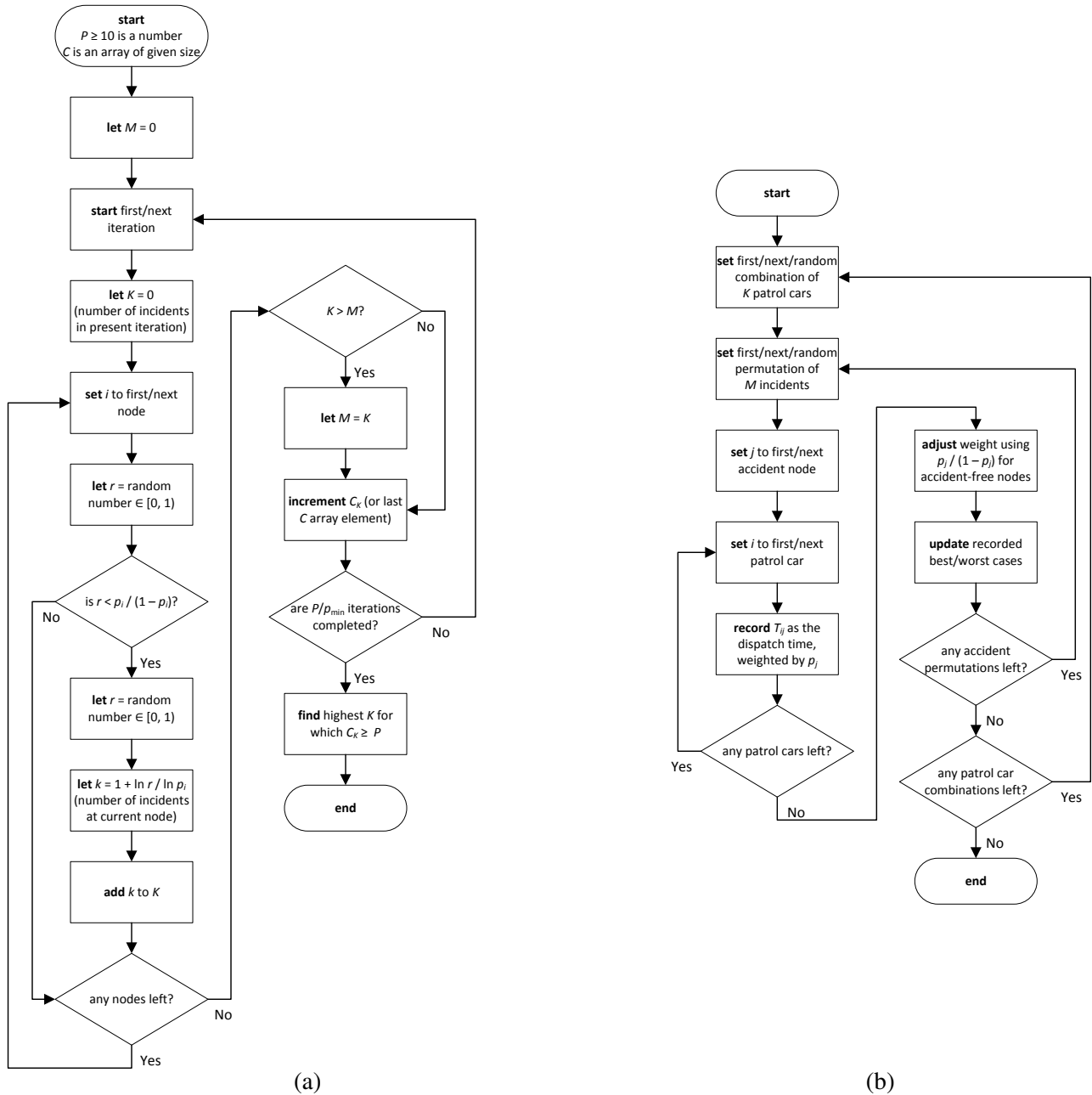
Fig. 2: (a) Algorithm to determine the maximum number of simultaneous incidents at a given probability. (b) Brute force method to enumerate all accident combinations.
