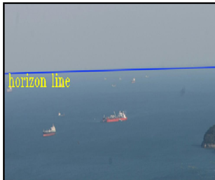
Fig. 5: Horizontal line detection by using ROI.
