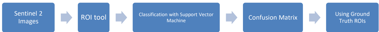
Fig. 4: Flowchart methodology of land cover mapping classification using the Sentinel 2A images with Support Vector Machine (SVM) in ENVI software.
