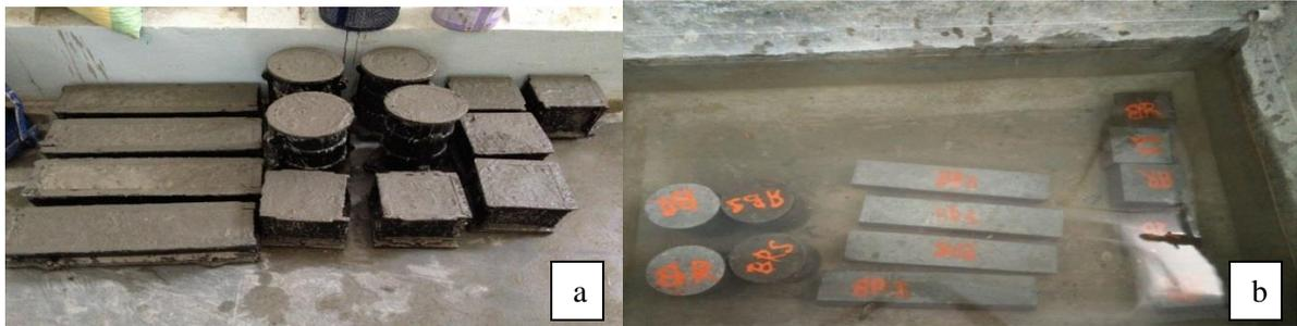
Fig. 2: (a) Casted concrete moulds (b) Water curing of concrete samples.
