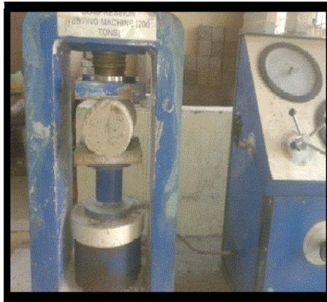
Fig. 7: Test on concrete cylinders for splitting strength
