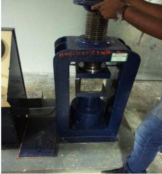
Fig. 3: Test on concrete cubes for compressive strength.
