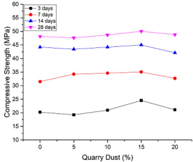
Fig. 4: Trend of compressive strength with quarry dust and steel slag.
