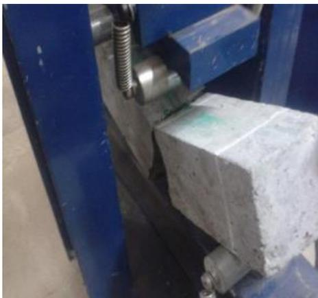
Fig. 5: Test on concrete beams for flexural strength.
