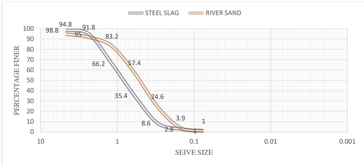
Fig. 1: Grain size distribution of steel slag and river sand.
