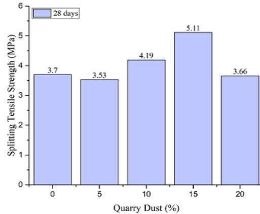
Fig. 8: Splitting tensile strength with quarry dust and steel slag
