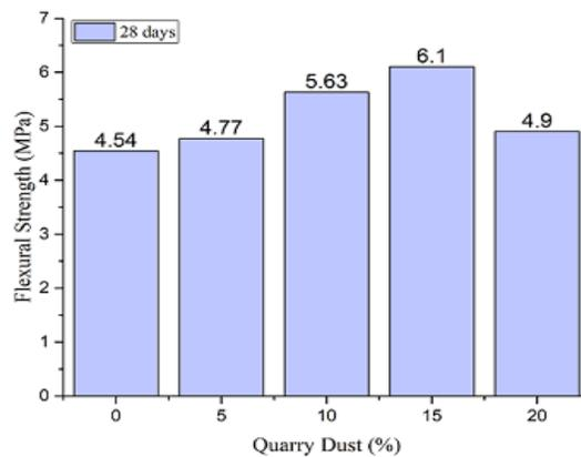
Fig. 6: Flexural strength with quarry dust and steel slag.
