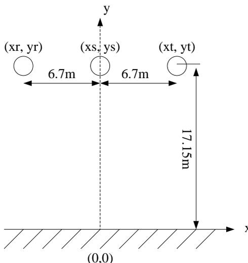
Fig. 1: Cross-section of 154 kV energy power transmission lines.
