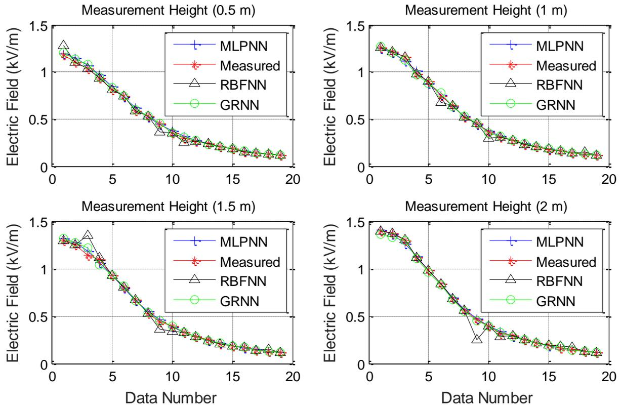
Fig. 2: Predicted Electric Field Intensity Values at Different Heights Obtained with 3 different artificial neural network algorithms (MLPNN, RBFNN & GRNN Methods) and Measured Values.
