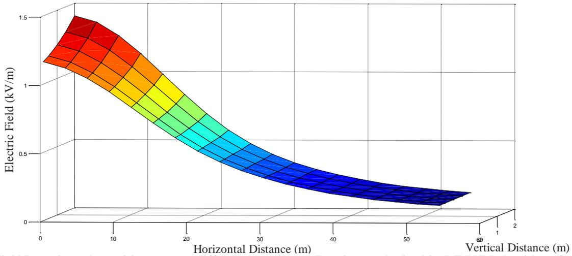
Fig. 3: Electric Field Intensity values with respect to different coordinates. Results are obtained by MLPNN algorithms for different heights.
