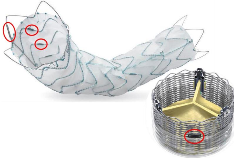
Fig. 1: Nitinol wires joined by crimping in a stent graft (Talent® Thoracic Stent Graft, Medtronic) and in a transcatheter heart valve (Lotus™ Valve, Boston Scientific Corporation). The crimping sleeves are indicated by the circles.
