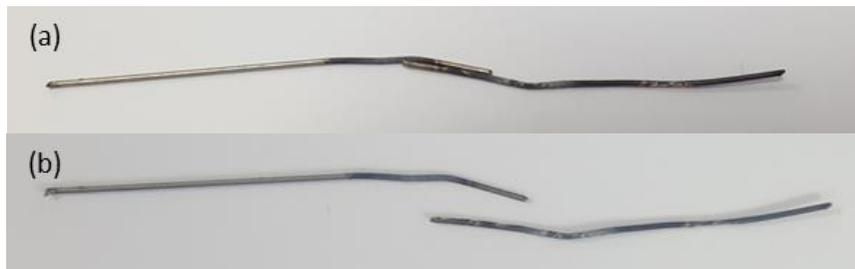
Fig. 4: (a) Resistance discharge welded nitinol wires, and (b) broken welds.
