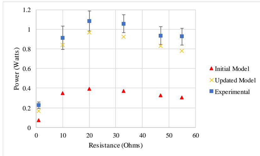
Fig. 4: PSpice power versus average prototype collected experimental data.
