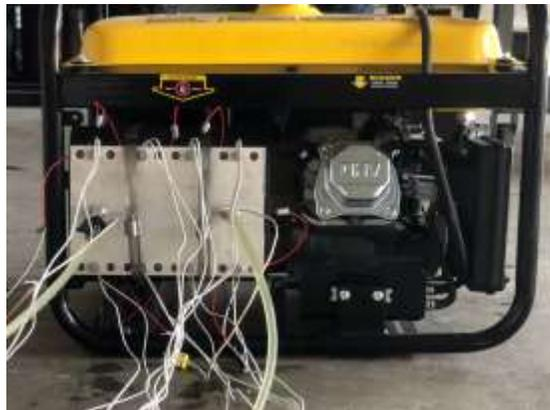
Fig. 3. Thermoelectric generator waste heat harvesting prototype mounted to muffler of generator.
