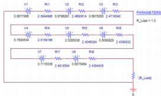
Fig. 2: Thermoelectric generator module in series.
