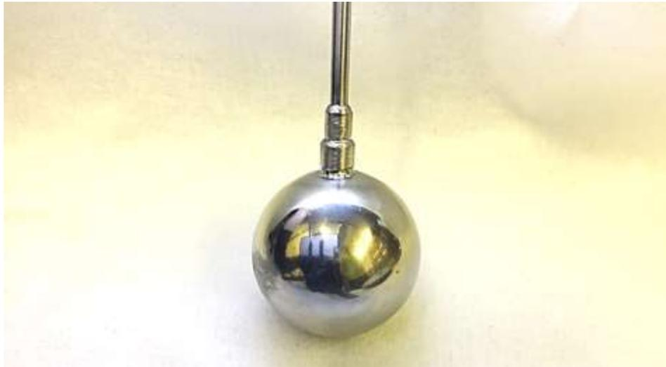
Fig. 3: Photo of stainless steel working sample with polished surface.
