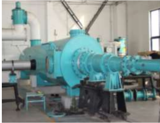
Fig. 1: FD-20 piston gun wind tunnel.
