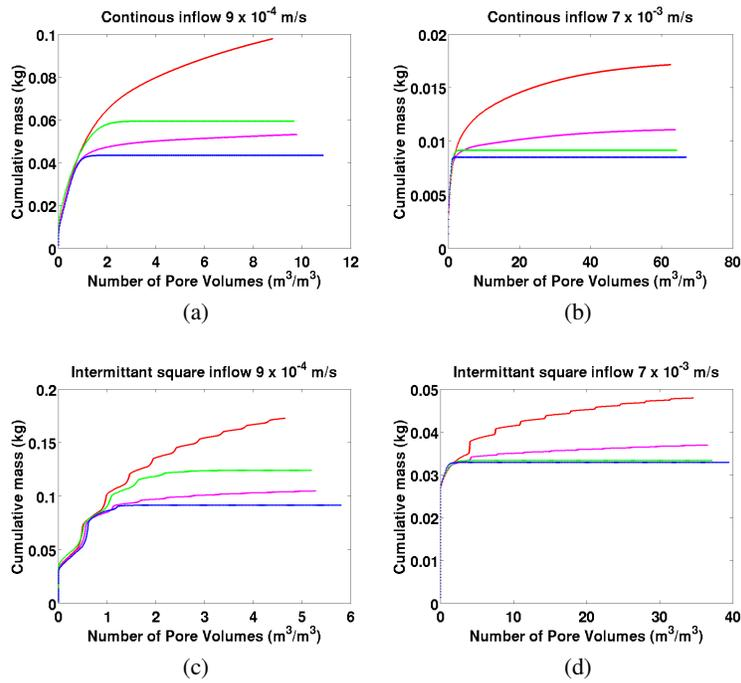
Fig. 4. Upscale discharge concentration mass against number of pore volumes for continuous ((a) and (b)) and intermittant square wave inflow infiltration((c) and (d)) at , and . Graph lines red (FM), magenta(SCP), green(SP), blue (H) indicate the spatial scenarios.
