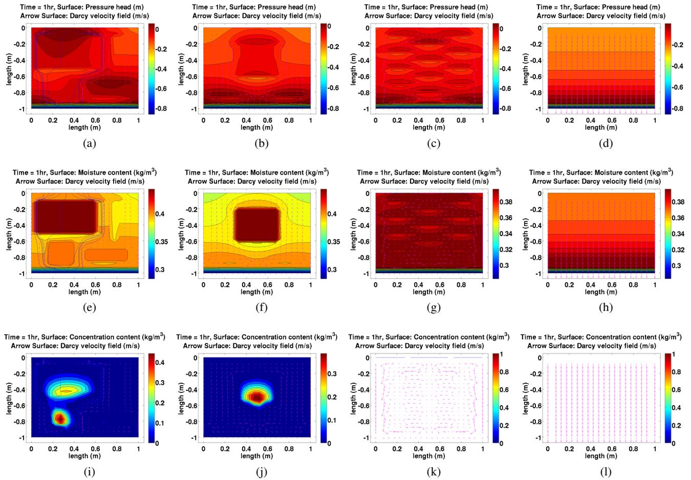
Fig. 3. Pressure head, moisture and concentration contents for different spatial scenarios for intermittent square wave inflow infiltration with rate of , at the end of 1.0 h.
