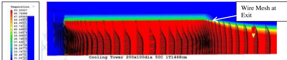
Fig. 4. Temperature profile shows reversal at exit fully blocked by the mesh.
