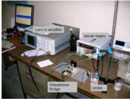
Fig. 2 Schematic diagram of 3\omega experimental set-up (Tavman and Turgut, 2010).
