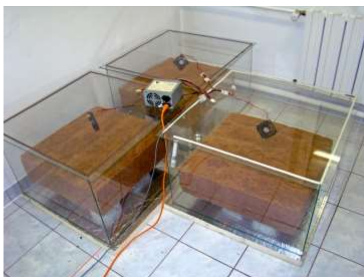
Photo 3. The conditioning chambers with wood wool samples.
