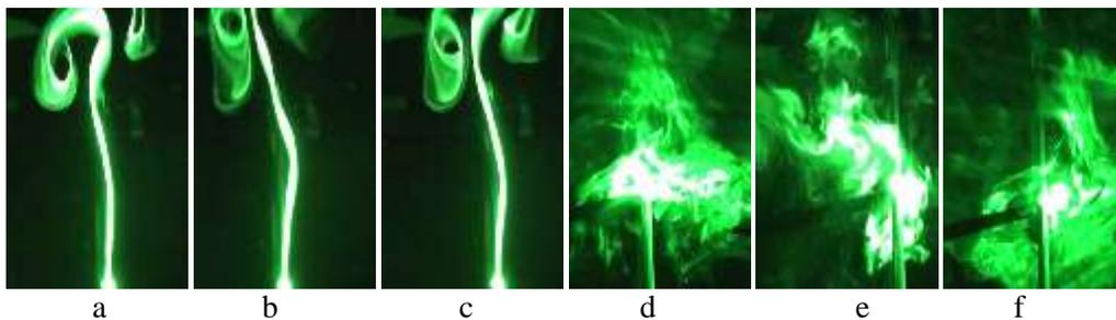
Fig. 9. Laminar plumes with transition region for the thick wire,  $Q=305$  W/m, quiescent environment (a,b,c) and the subsequent effect of turbulence with  $u_{RMS} = 0.78$  m/s (d,e,f)
