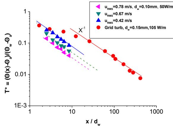
Fig. 8. Distribution of dimensionless centerline temperature in the  $x$  direction for the thin wire,  $d_w=0.10$  mm,  $Q=50$  W/m. Comparison with exp. result in grid turbulence,  $d_w=0.15$  mm,  $Q=105$  W/m, Stapountzis et al (1986)
