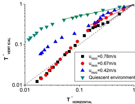
Fig. 7. Comparison of dimensionless centerline temperatures in the horizontal and vertical directions for the same values of  $x$  and  $z$  coordinates, thick wire,  $Q=305\text{ W/m}$
