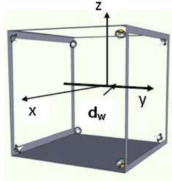
Fig. 1. Turbulence Chamber with eight loudspeakers for the generation of Synthetic Jet Turbulence and coordinate system used. The heated line source is along the y direction.
