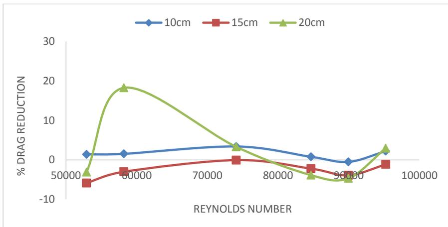
Fig. 5. Relationship between percentage of drag reduction and Reynolds number and with different length of mechanical device of 10cm, 15cm and 20cm on 2m pipe.
