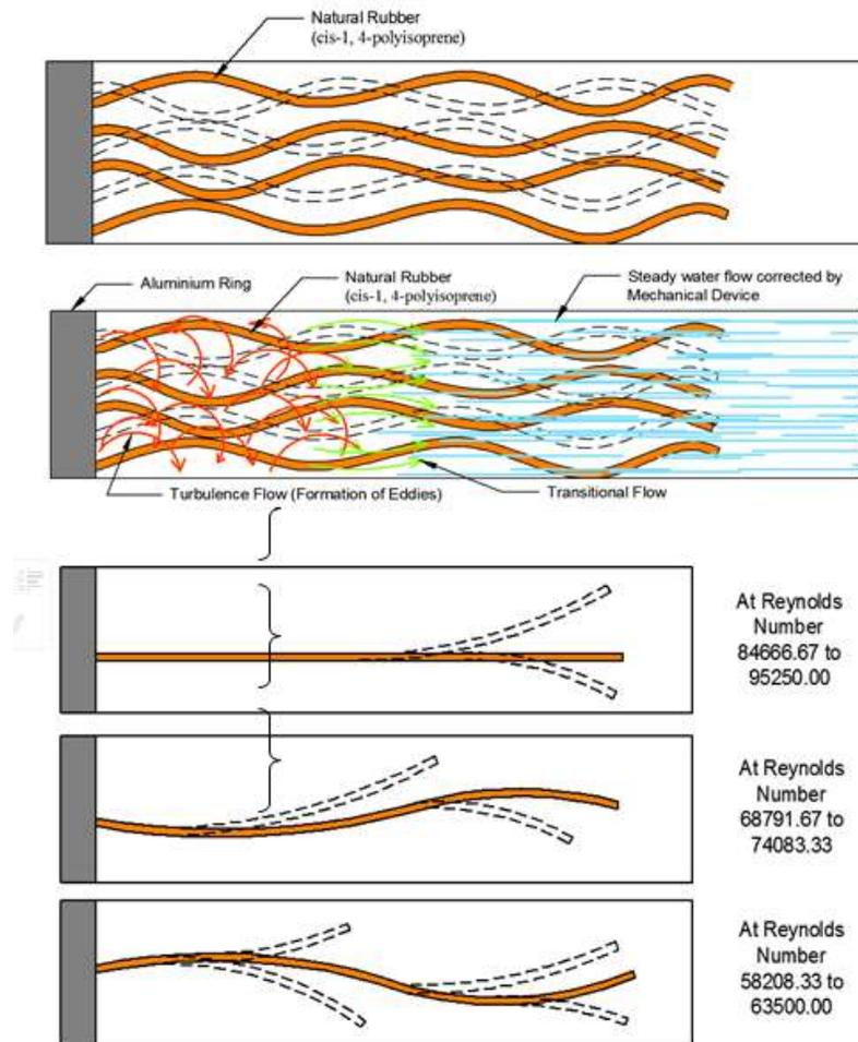
Fig. 8. The mechanism of water flow in pipeline with the presence of mechanical device.
