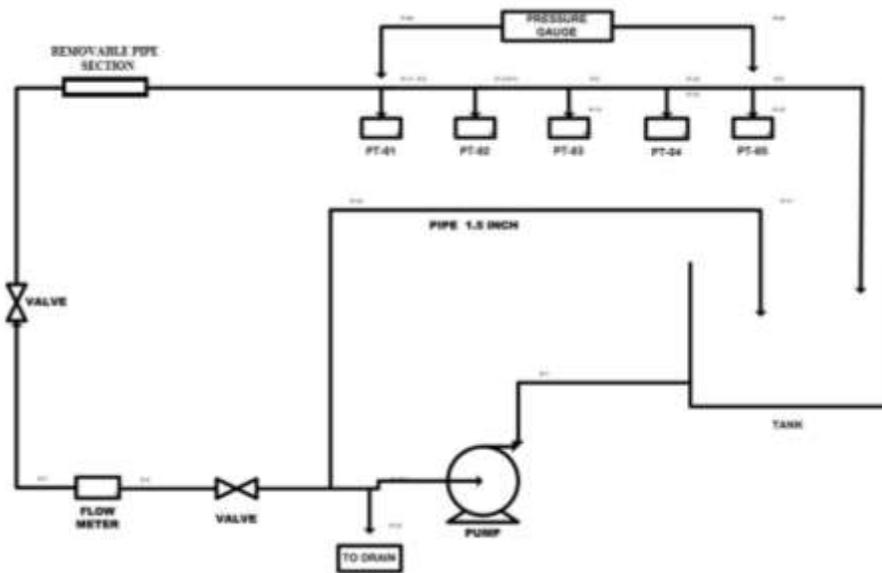
Fig. 1. Closed-Loop Circulation Rig.
