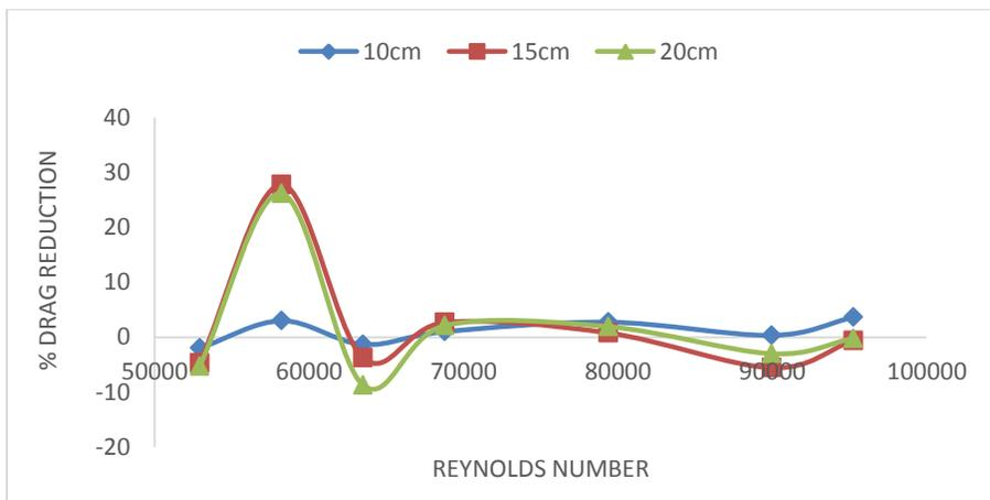
Fig. 6. Relationship between percentage of drag reduction and Reynolds number and with different length of mechanical device of 10cm, 15cm and 20cm on 1.5m pipe.
