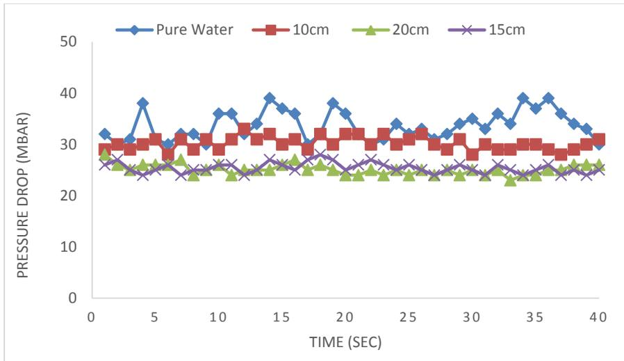
Fig. 4. Pressure drop influenced by the mechanical device of 10cm, 15cm and 20cm length on 0.5m pipe at  $Re = 95250.00$ .
