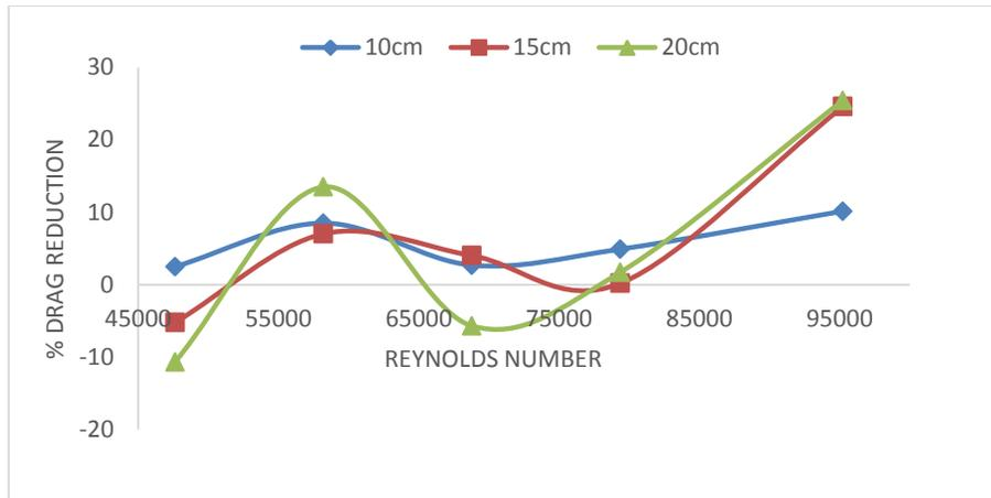
Fig. 7. Relationship between percentage of drag reduction and Reynolds number and with different length of mechanical device of 10cm, 15cm and 20cm on 0.5m pipe.
