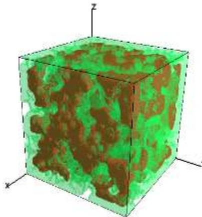
Fig. 1. Digital rock model of Berea sandstone: quartz – green color, feldspar – brown color.
