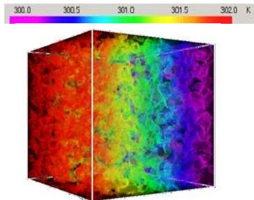
Fig. 2. Stationary temperature field of hydrophilic porous media (Berea sandstone) with water saturation  $S_w = 50\%$ .
