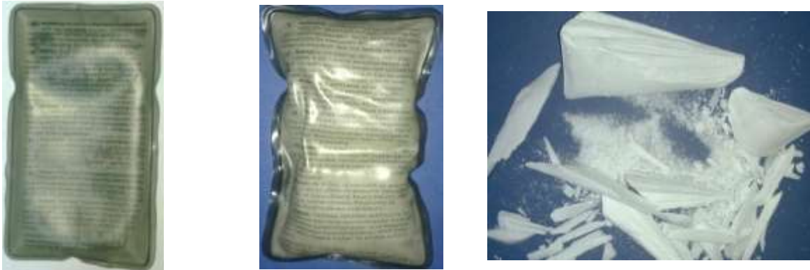
Fig. 1. Tested sample (prior to measurement – liquid in a PVC soft bag; on completion of the measurement – solid body in PVC; hydrated sodium acetate).
