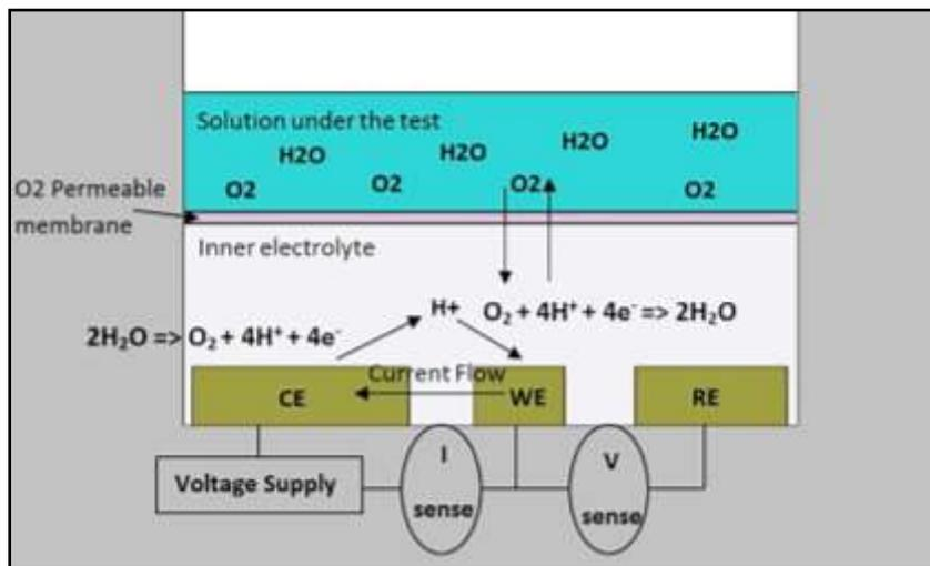
Fig. 1. Principle of oxygen sensor operation [redrawn from McLaughlin et al., 2005]
