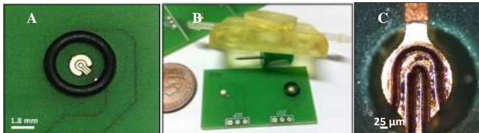
Fig. 5. A. The Ni/Au coated geometry of the Clark sensor fabricated on PCB. B. The primary cell culturing platform and the sensor platform is ready to assemble. C. Image of the 20  $\mu\text{m}$  WE after laser micro machining, captured by Alicona G4 Infinite Focus system.
