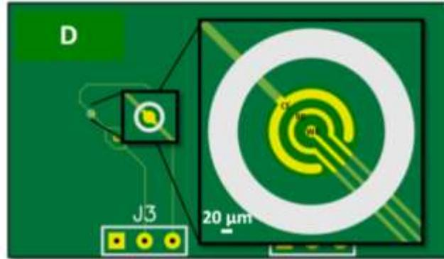
Fig. 3. Design of the sensor with 20 microns precision.
