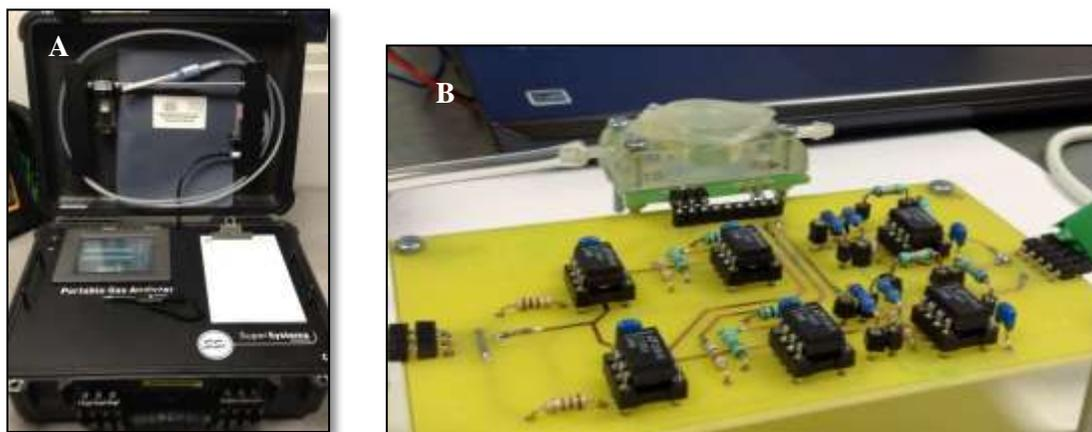
Fig. 6. A. Portable Gas Analyser 3510. B. The measurement circuit board with oxygen sensor platform
