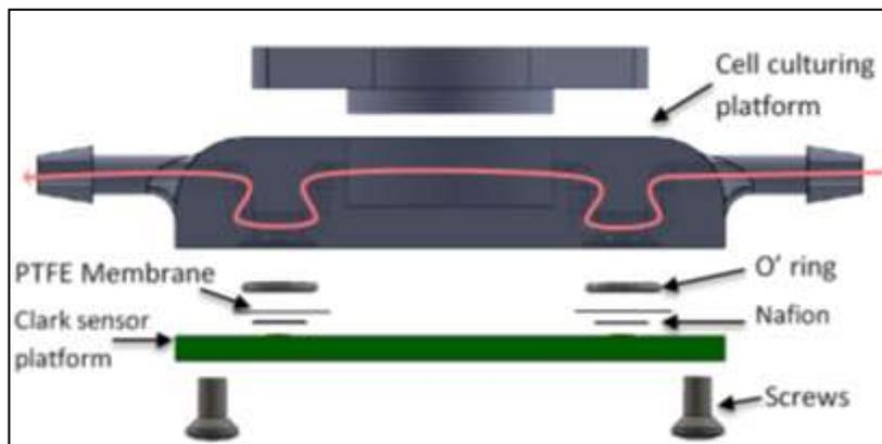
Fig. 4. Assembling the sensor platform and the cell culturing platform with Nafion electrolyte, PTFE membrane and O' rings.
