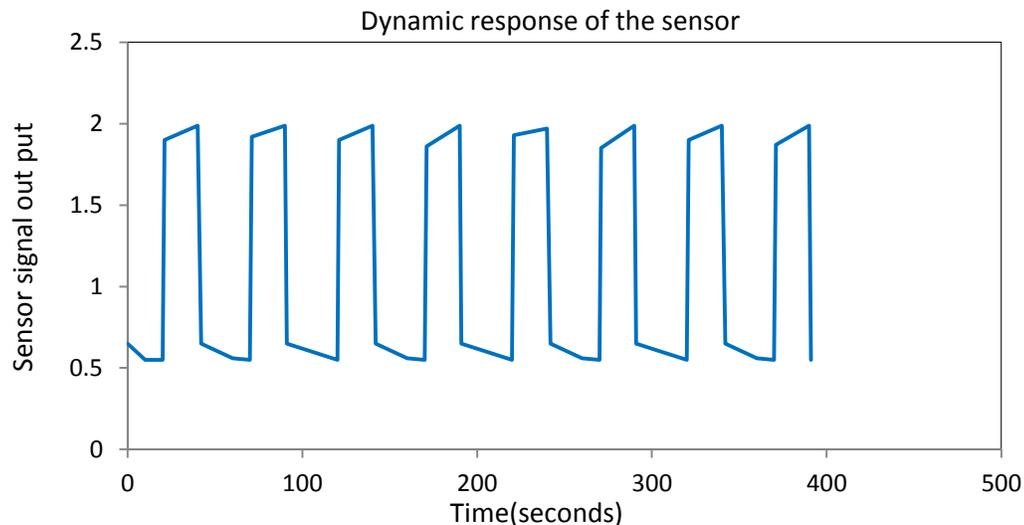
Fig. 8. Dynamic response of the WE having diameter of 300  $\mu\text{m}$  between 0% to 20% oxygen concentration.
