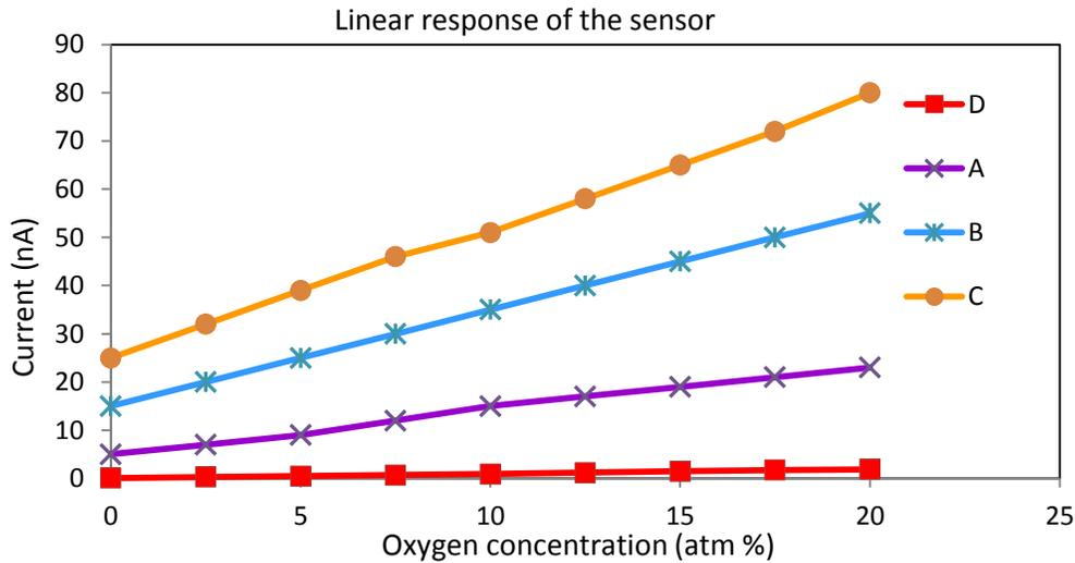
Fig. 7. Step linearity response of the WE having four different sizes between 0% to 20% oxygen concentrations.
