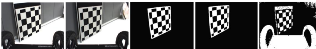
Fig. 6. The calibration target: the left and right CCD cameras (left), the TOF camera intensity image (center), the left and right thermal imagers (right) camera.
