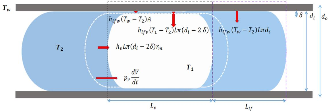
Figure 1: Schematic diagram of the system
