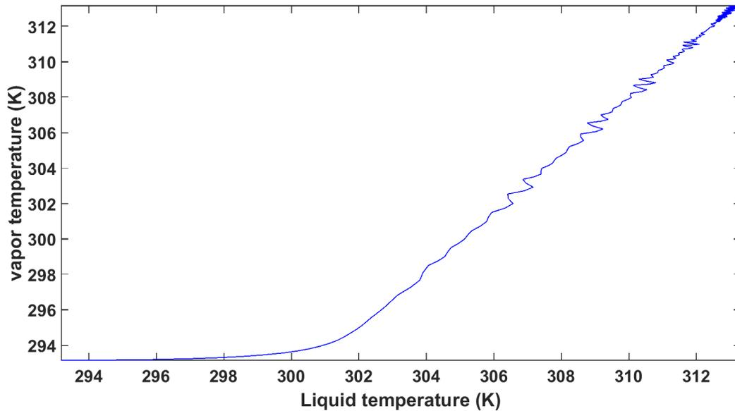
Figure 5: Phase portrait of the liquid slug temperature and the vapor plug temperature showing the thermal equilibria
