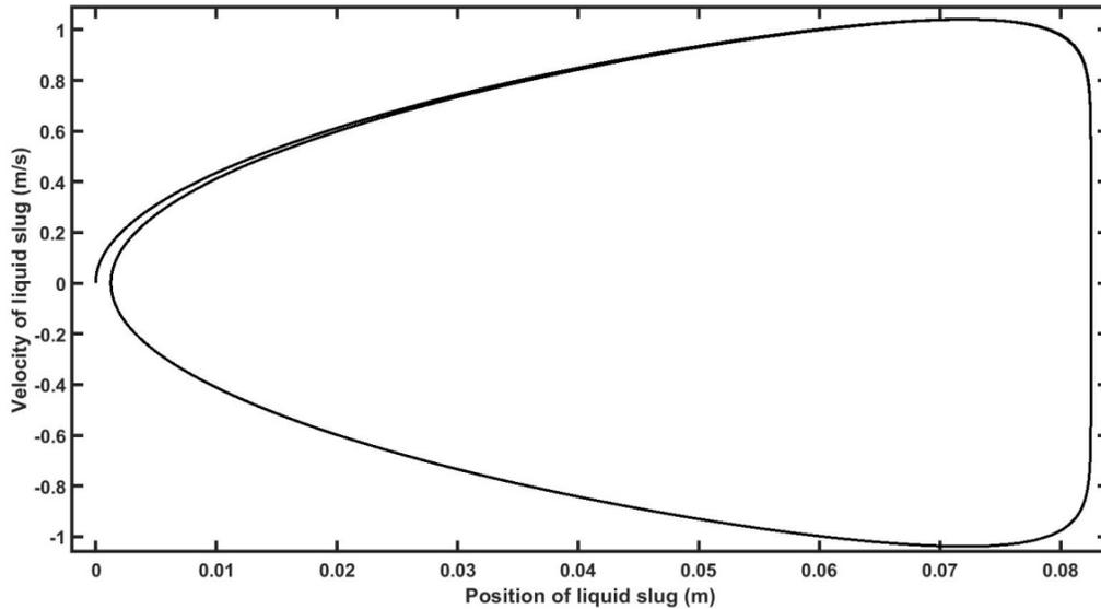
Figure 3: Phase-portrait of position and velocity of a liquid slug at  $h_{lfv} = 200 \text{ W/m}^2\text{K}$
