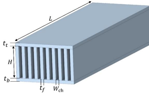
Fig. 1: Schematic of the heat sink.
