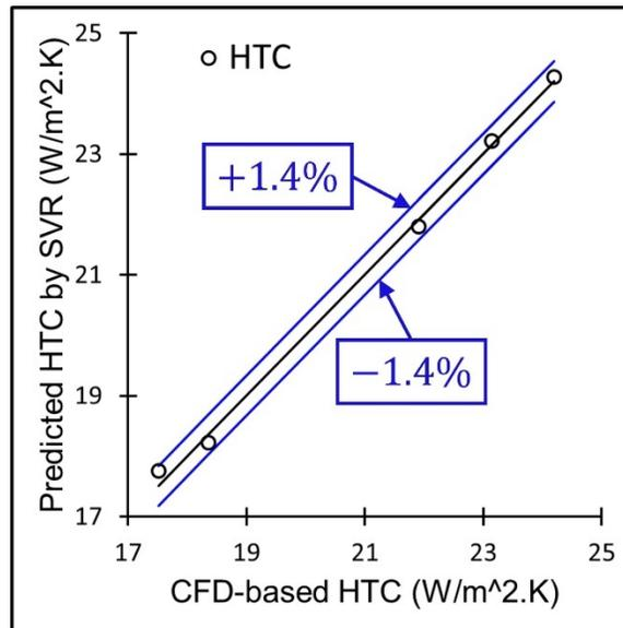
Fig. 2: Comparison between predicted HTC by SVR approach and CFD-based HTC.
