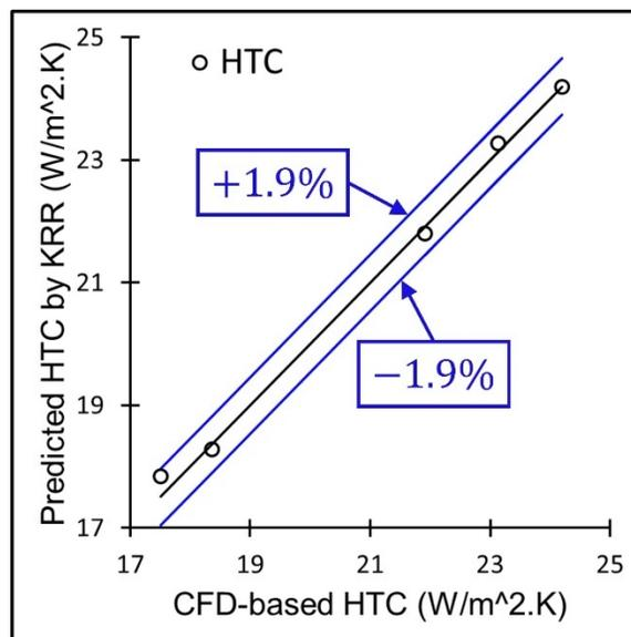
Fig. 3: Comparison between predicted HTC by KRR approach and CFD-based HTC.
