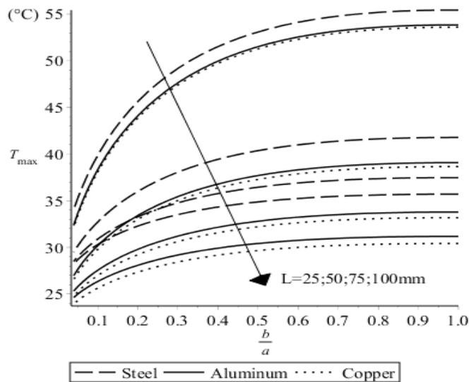
Fig. 3: The maximum temperature as a function of the ratio between the semiminor and semimajor axes of the ellipse for the three materials and different lengths in the case of forced convection.
