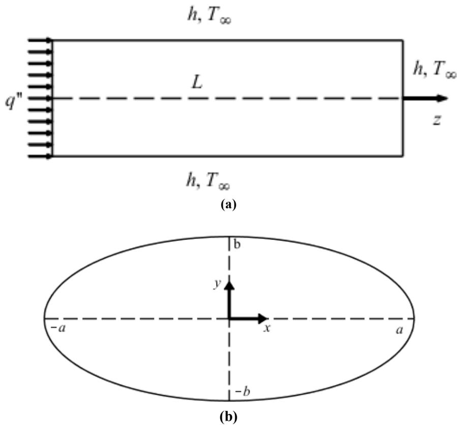
Fig. 1: The geometrical configuration of the uniform fin: (a) Side-view, (b) Elliptical cross-sectional shape.
