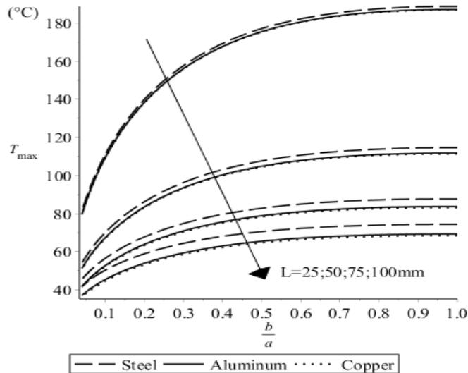
Fig. 2: The maximum temperature as a function of the ratio between the semiminor and semimajor axes of the ellipse for the three materials and different lengths in the case of natural convection.
