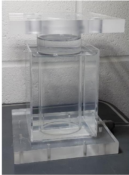
Fig. 5: Experimental bubble column reactor investigated by Chen and Brooks. (Chen and Brooks [31]).
