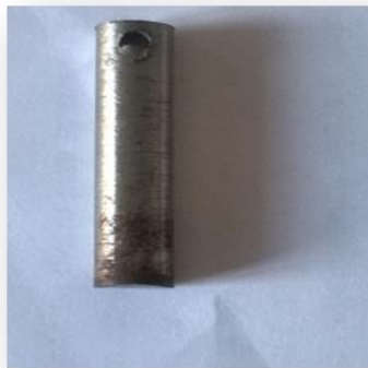
Figure1: Preparing of the sample for the weight loss measurements
