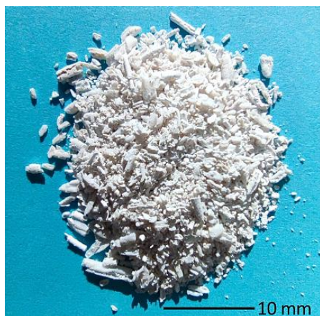
Fig. 3: Condensate from the roasting of industrial copper telluride
