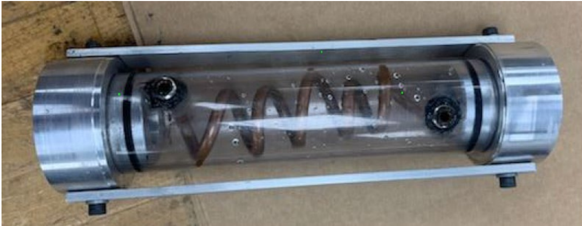
Fig. 2. Heat exchanger HE-1
