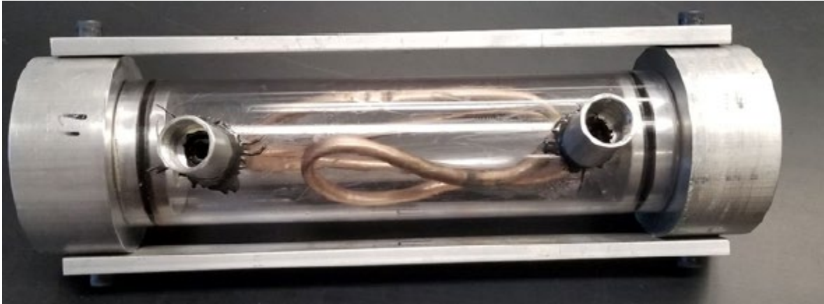
Fig. 4. Heat exchanger HE-3
