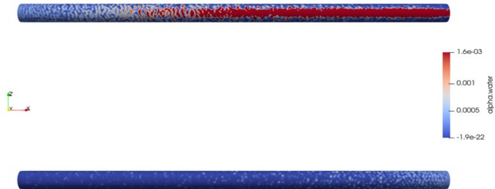
Fig. 5: Distribution of the aqueous phase on the pipe walls
