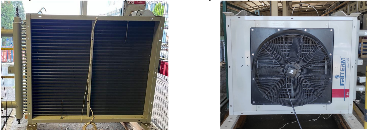
Fig. 1: The heat exchanger to be tested
