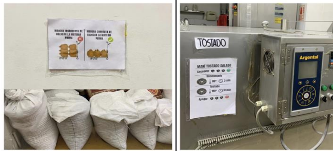
Fig. 9: Implementation of the Poka Yoke Informative type 1 and 2
