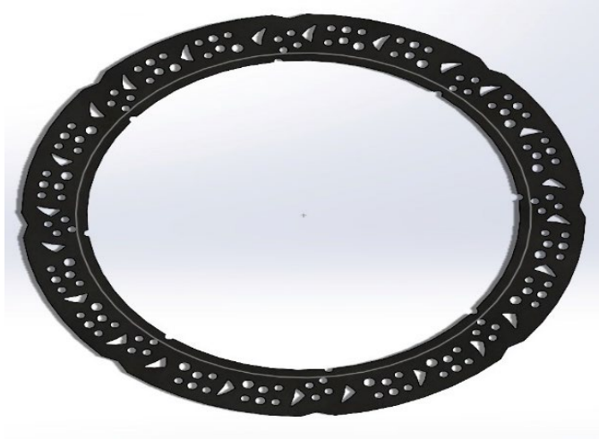
Figure 4: Extruded brake rotor used for the thermal analysis.
