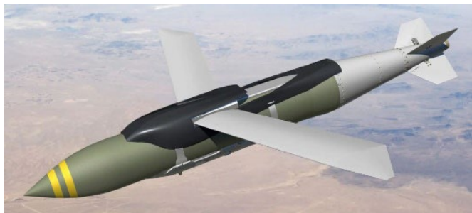
Fig. 2: Examples of expandable wings for munitions; JDAM-ER by Boeing [9]
