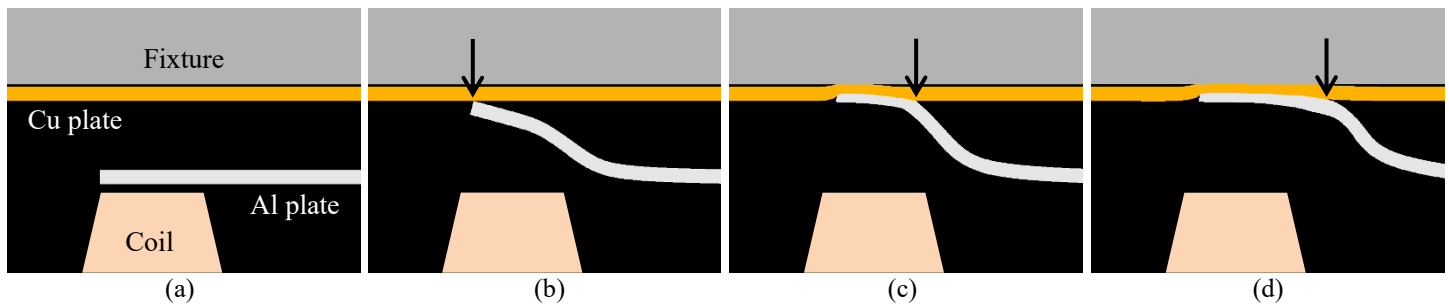
Fig. 4 Deformation and collision behavior of the plates. (a) Before welding. (b) Initial collision. (c) 2 \mu s after initial collision. (d) After welding.
