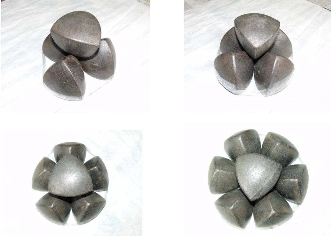
Fig.4. Possible arrangement of the Relo body in two layers
