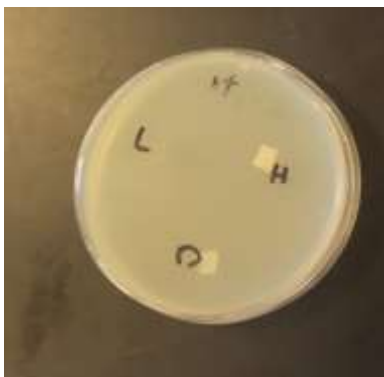
Fig. 3: Antibacterial testing of the fibers containing silver nanospheres against wild type E. coli . The samples are labelled as L (control sample), H (ampicillin-loaded fibers) and D (ampicillin soaked sample).
