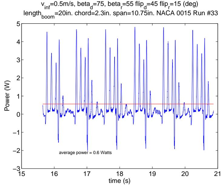
Fig. 7. Left plot shows that the dynamic response of the DC generator is significantly different from the linear steady-state response. The right plot show that the average cycle power for this run was 0.6 Watts.
