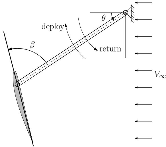
Fig. 1. Top view of hydrofoil and boom arrangement. The clockwise rotation to the side is the deploy stroke and the counter-clockwise rotation is the return stroke.
