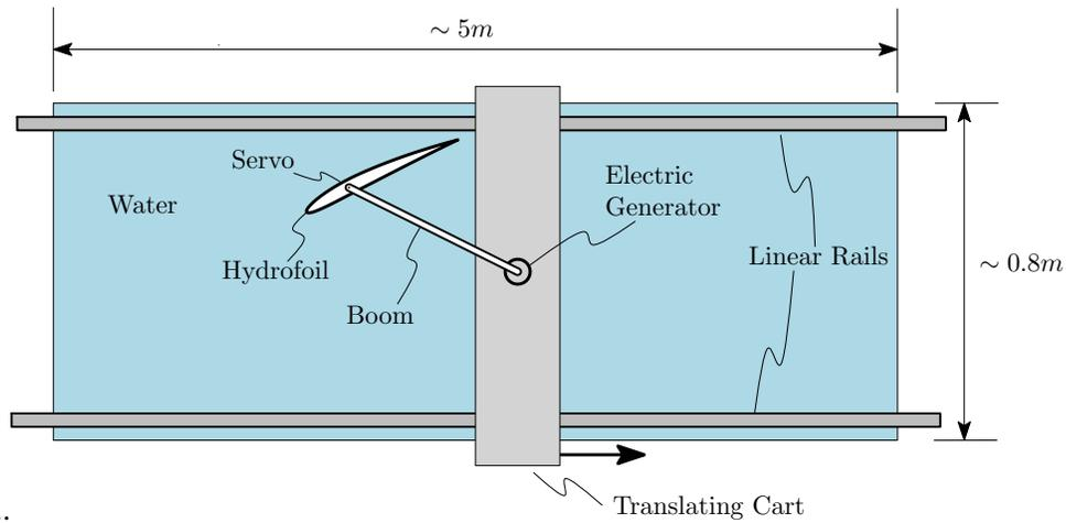
Fig. 2. Top view schematic of the tow-tank with small-scale hydrokite system used for the experiments.
