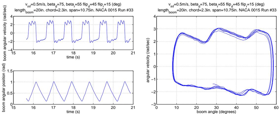
Fig. 5. Left plot shows the angular position of the boom along with the calculated time derivative of that signal. The right plot shows a phase plane plot of the periodic boom motion.
