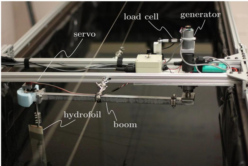
Fig. 3. The figure shows the boom and hydrofoil connections in the tank along with the load cell used to measure the forces, the generator, the encoder and the dump load. The system is present in the Energy and Motion Laboratory, Rochester Institute of Technology, Rochester.
