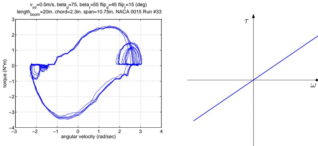
Fig. 6. Left plot shows that the dynamic response of the DC generator is significantly different from the linear steady-state response. The right plot shows a standard simplified steady-state generator response for a DC motor.
