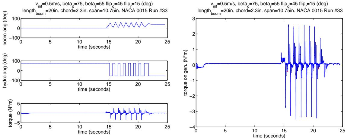
Fig. 4. Left plot shows the raw position and torque data collected from the sensors along with the desired hydrofoil angle. The two red marks delineate the clipped data which isolates the stable periodic motion of the system and ignores the data from the transient portions of the motion.
