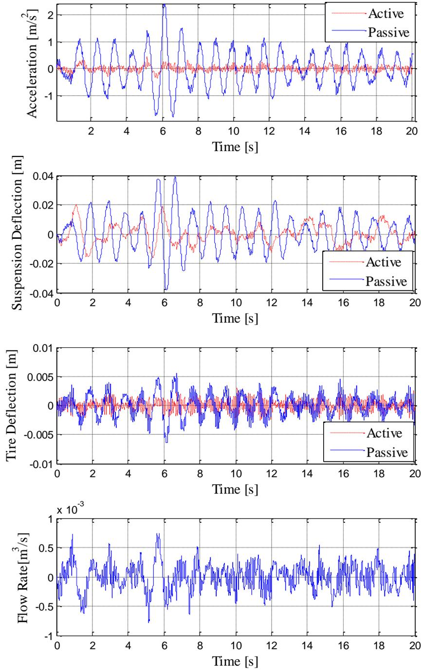
Fig. 6. Simulation results for random road displacement input for active and passive suspension.
