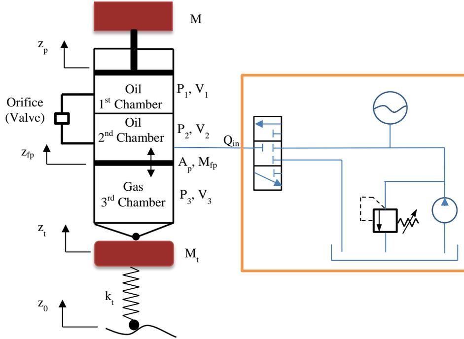
Fig. 1. Active HP suspension.
