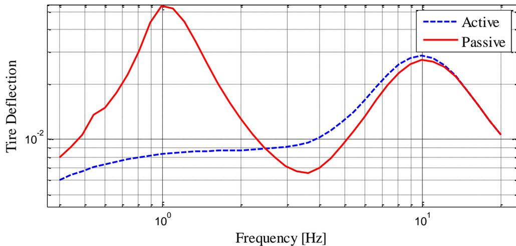
Fig. 4. Tire deflection FRF for passive and active HP suspension.
