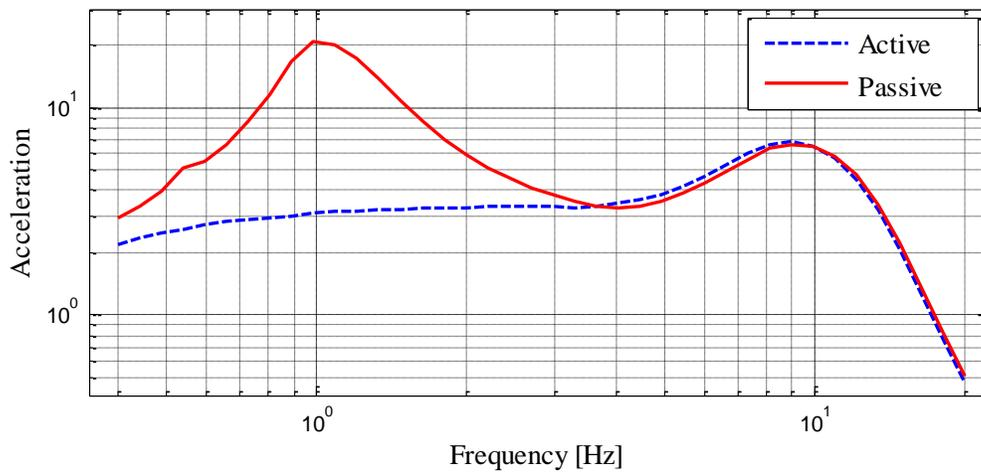
Fig. 2. Sprung mass acceleration FRF for passive and active HP suspension.
