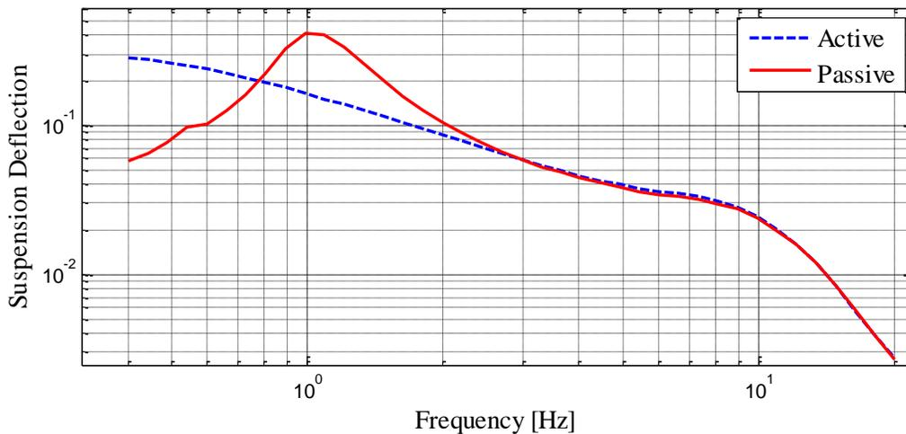
Fig. 3. Suspension deflection FRF for passive and active HP suspension.
