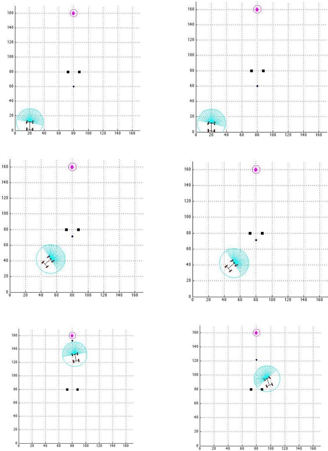
Fig. 6 Six frames of the simulation of a non-holonomic robot following a human while avoiding obstacles.
