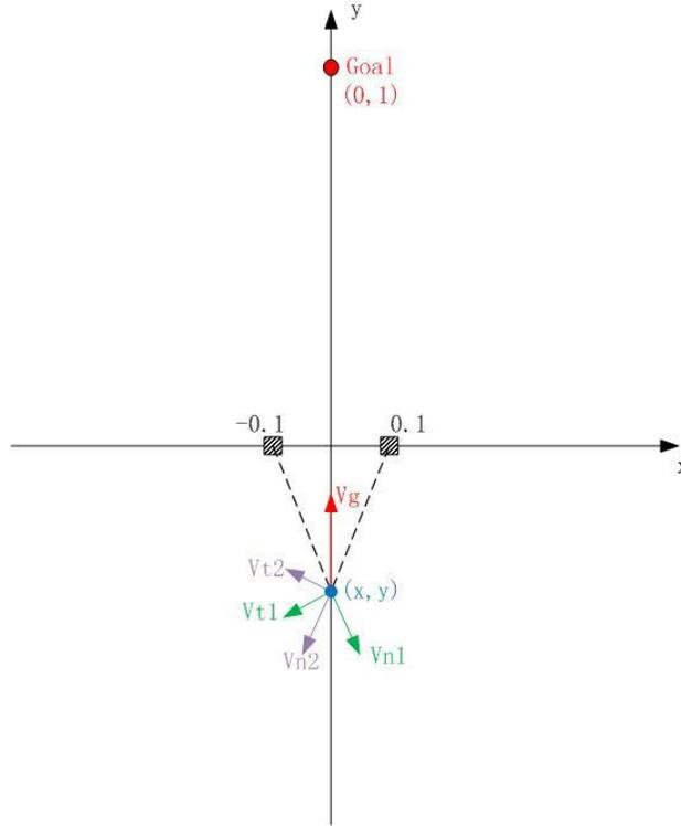
Fig. 1. Position of obstacles and goal and velocity commands of robot.
