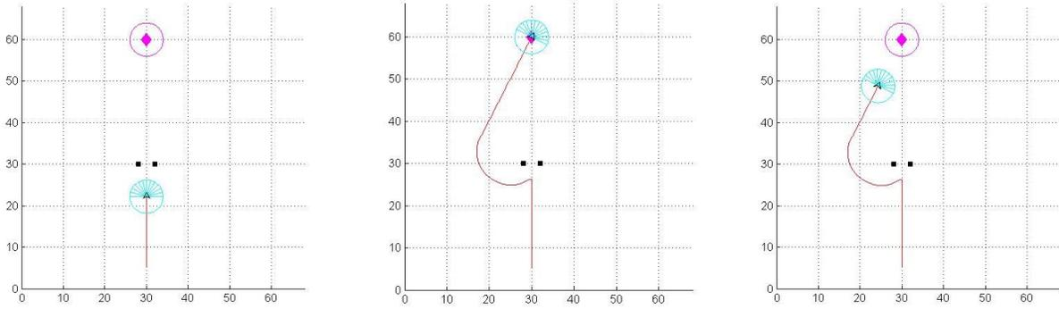
Fig. 4. Three frames of the quasi-harmonic function simulation results for a robot avoiding two obstacles [11].
