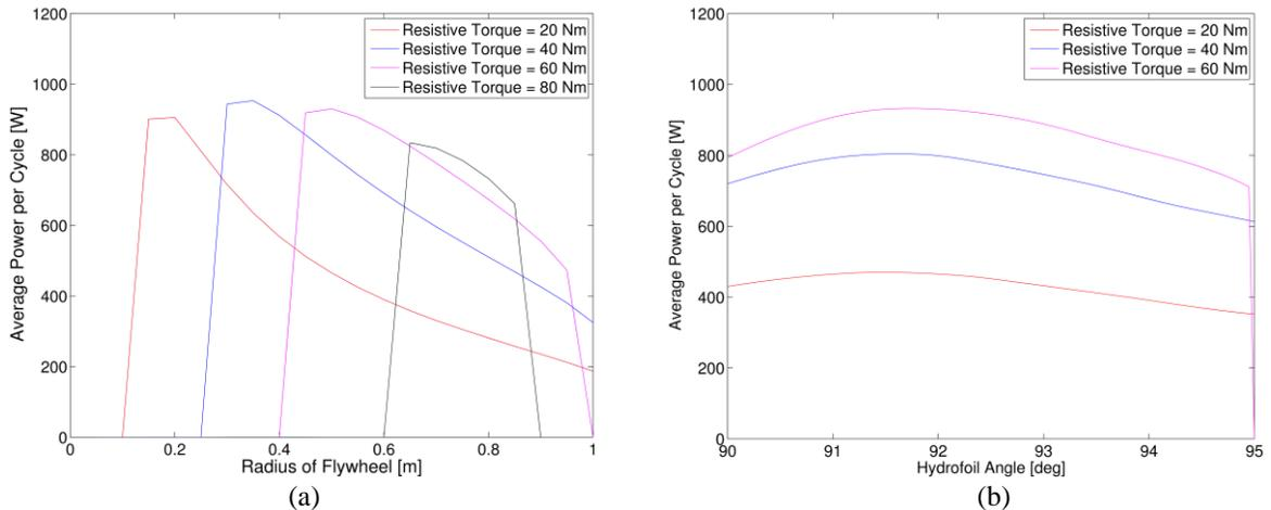
Fig. 3 (a&b) Average cycle power as a function of (a) Flywheel radius and (b) Hydrofoil angle for several braking torques
