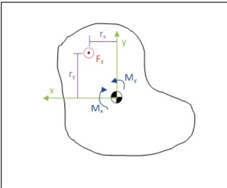
Fig. 1. Normal force location to counteract the tipping moments on the block model with a generic footprint
