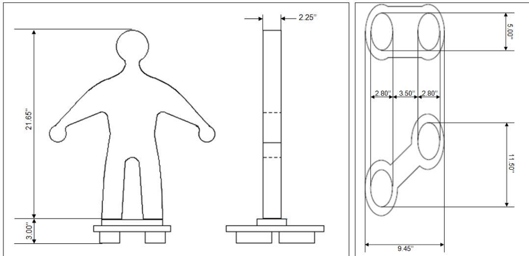
Fig. 2. Scaled drawing of the MII man assembled apparatus with staggered footprint attached and the straight and staggered footprint configurations.
