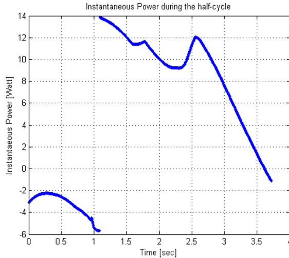
Fig. 6. Instantaneous power decreases with time in the reel-out phase.
