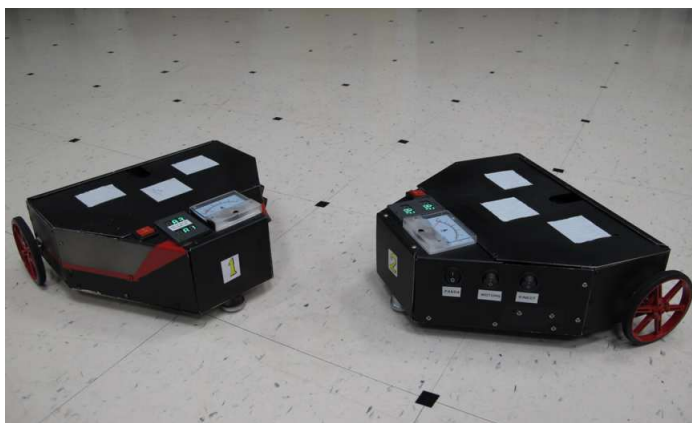
Fig. 3. Experimental differential drive wheeled mobile robots.
