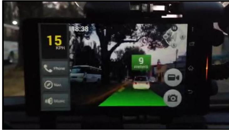
Fig. 2: Measurement of velocity of the instrumented car and of the distance to the car in front of it (IonRoad App V 1.6.3 Pro is a license of iOnRoad Limited [25]).
