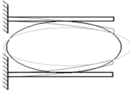
Fig. 2: Two set micro-cantilever beams with a droplet between them.
