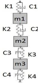
Fig. 1: The schematic view of a mass-spring-damper system of twin micro-cantilever beams with a droplet between them.
