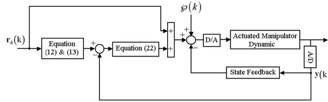
Fig. 1: Model free digital feed forward control scheme.
