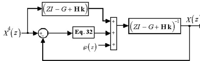
Fig. 2: Equivalent form of Model free digital feed forward control scheme.
