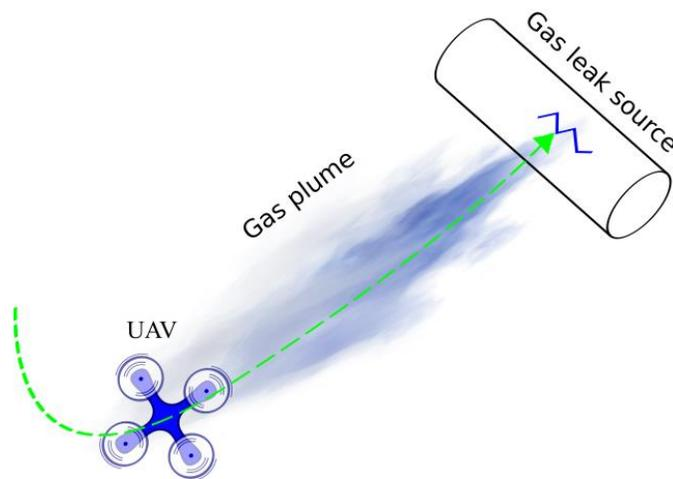
Fig. 1: Shows the UAV traveling towards the gas plume to localize the gas source leak.
