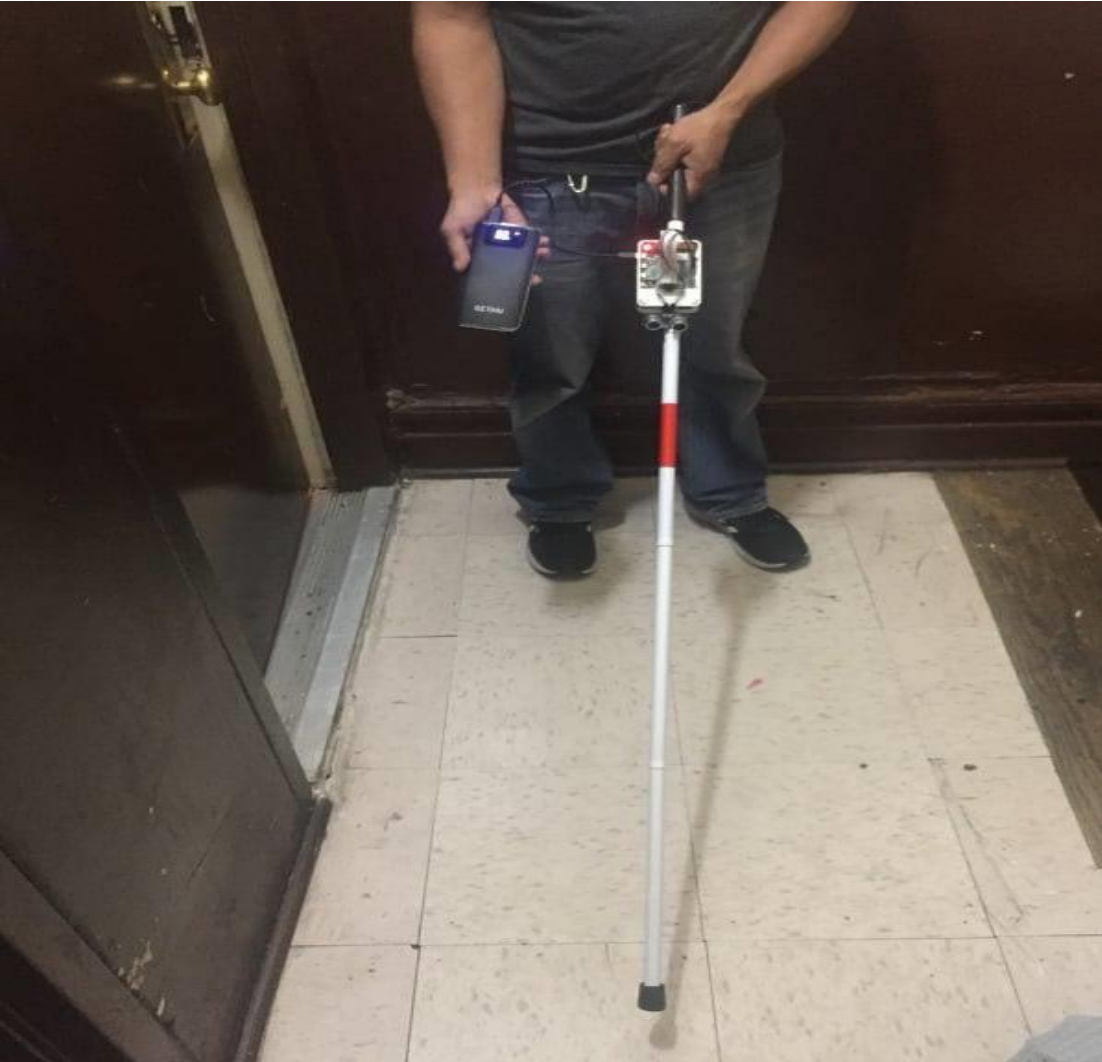
Fig. 8: Camera and Sensor Attached to White Cane.
