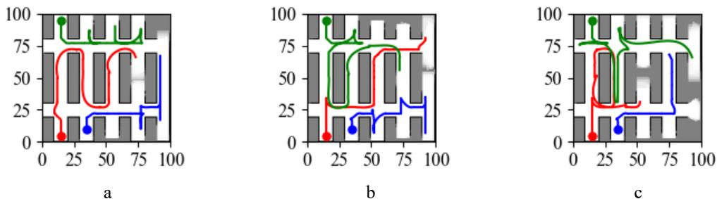
Figure 5. Effects of the anti-pheromone mechanism: a. with anti-pheromone mechanism and 90% map coverage, b. without anti-pheromone mechanism and 90% of coverage; the exploration time is more than (a), c. without anti-pheromone mechanism and the same time as (a).
