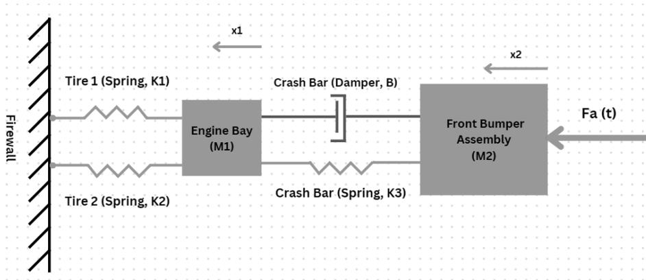
Fig. 1: Overall system diagram
