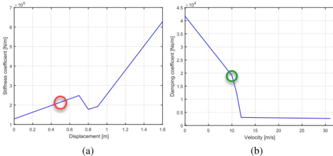
Fig 3: Spring and damper forces of a vehicle chassis during a crash [6].
