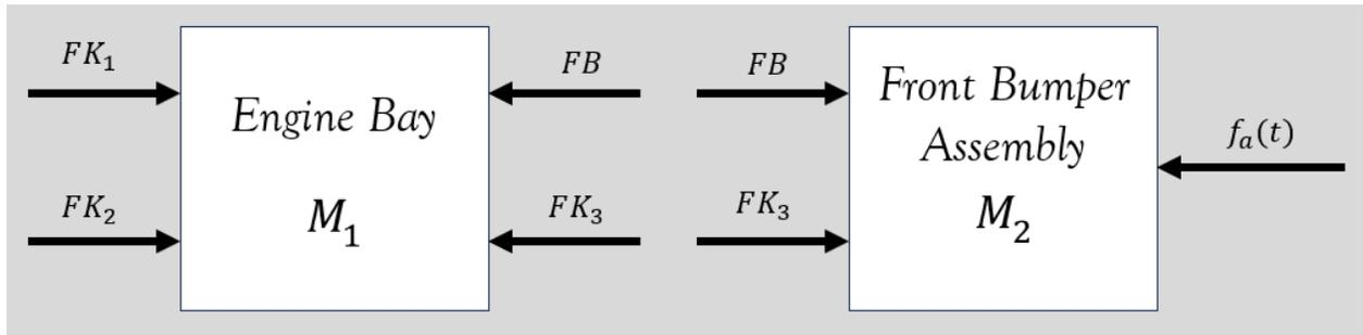
Fig 2: Free body diagram showing forces acting on each mass.
