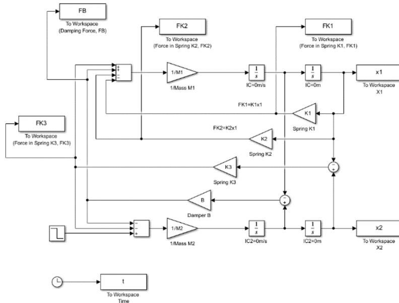
Fig 5: Simulink model created for Matlab representation of the system.
